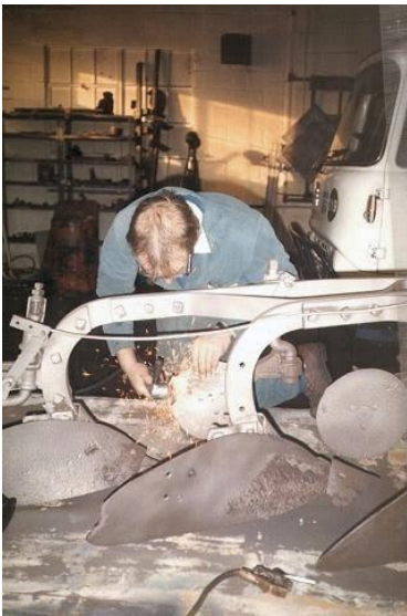
After shot-blasting to remove the rust, the rough edges are tidied up a bit by a member of Edgehills' staff.
